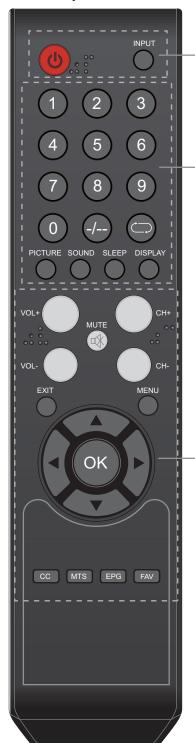
**OPENICATION** POWER(red button): Turn the TV on/standby. INPUT: Press to display the input source menu.
